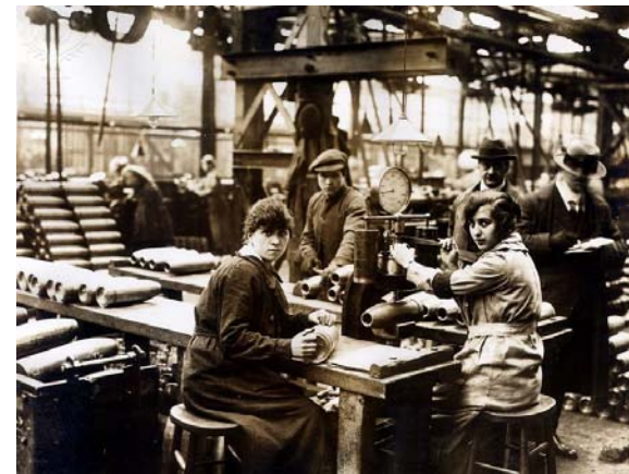
Caption: World War One - munition factory making shells, women weighing steel shells and testing their hardness. April 1918 Credit: Mirrorpix / Universal Images Group Copyright Notice: Copyright Universal Images Group
