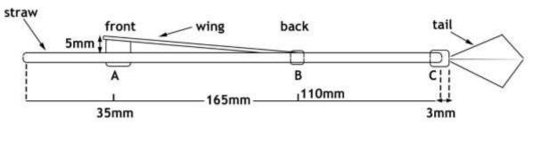
Finished glider (Not to scale) Trying to fly: making a model of Cayley's glider -
